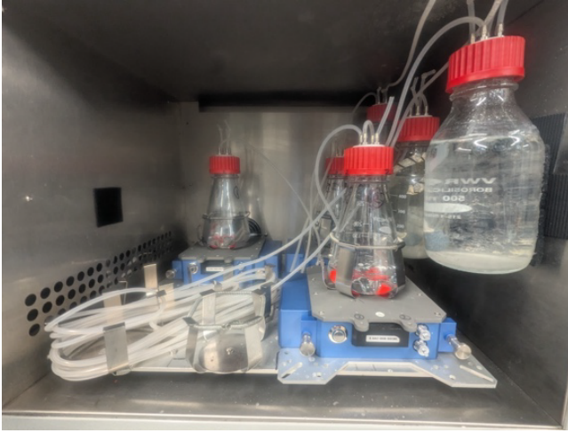
Figure 1. Photograph of experimental set-up. The blue base units are the PreSens Shake Flask Readers. The media bottles visible on the right humidify the enriched air before it enters the baffled flasks.
