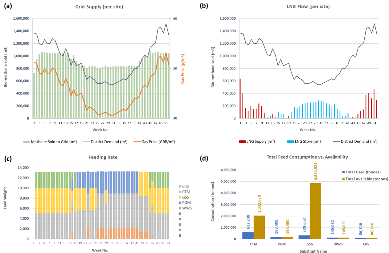
Figure 2. Operational performance – Type A plant (Inverness): (a) production vs demand; (b) LNG schedule; (c) blend ratios; (d) feed availability/use.
