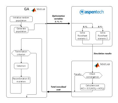
Figure 3: The solution algorithm combines a genetic algorithm in Matlab with the process simulator ASPEN Plus.
