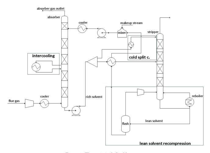
Figure 4: The optimized, flexible process.
