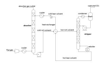
Figure 1: Conventional MEA-based absorption process [7].
