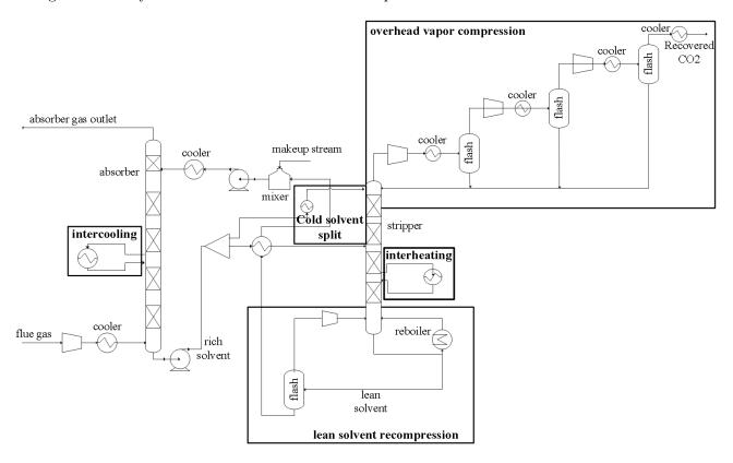
Figure 2: CO<sub>2</sub> capture process flowsheet with all configuration included.
