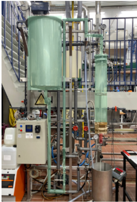
Figure 1: (Left) An image of the pilot-scale fixed-bed ion exchange column and (right) P&I diagram for the pilot-scale ion exchange fixed-bed column [8]. The green, orange, and red sections on both the image and the P&I diagram represent the in-flow pipes, the fixed-bed column, and the out-flow pipes, respectively.
