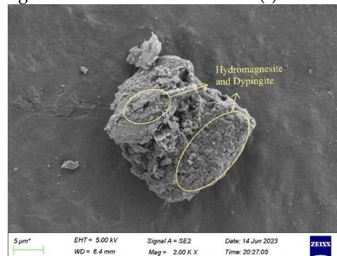
(g) Silt + 9% \text{MgO} + \text{CO}_2 .
