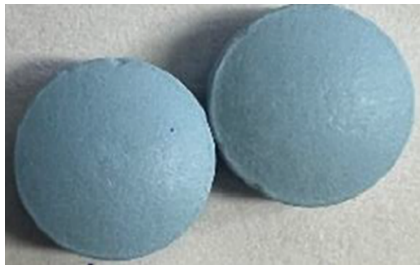
Figure 1. Tablet edge damage defects
