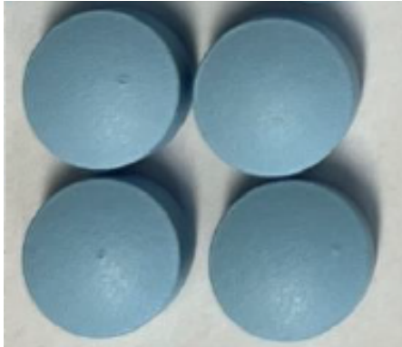
Figure 1. Tablet edge damage defects
