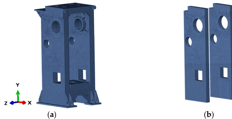
Figure 8. Model for topology optimisation: (a) complete finite element model; (b) design domain.
