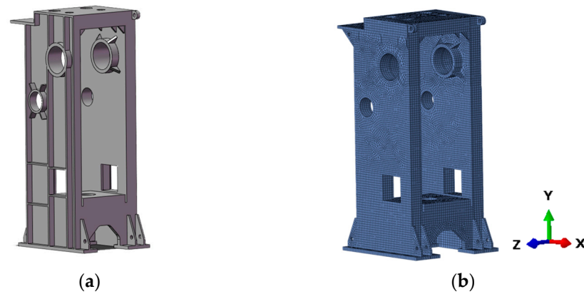
Figure 4. Modelling of the press frame: (a) three-dimensional solid model; (b) finite element model.
