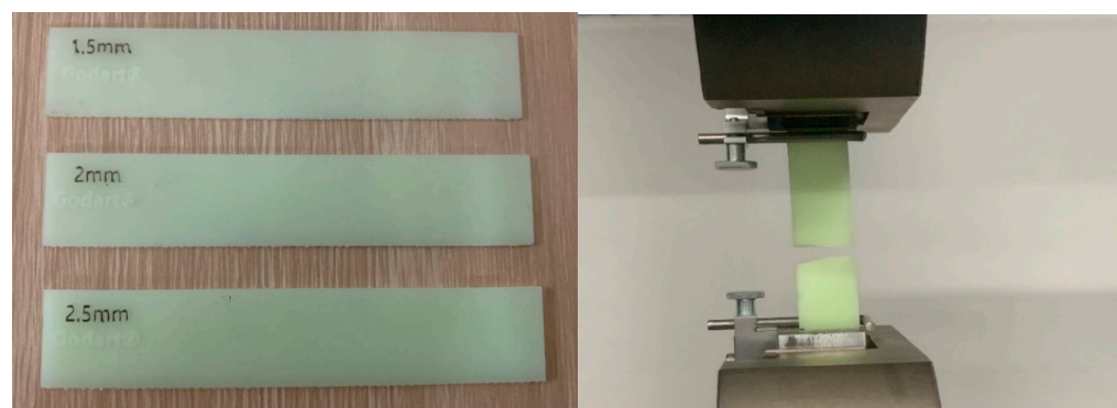
Figure 13. The 8228 resin specimens' tensile test.
