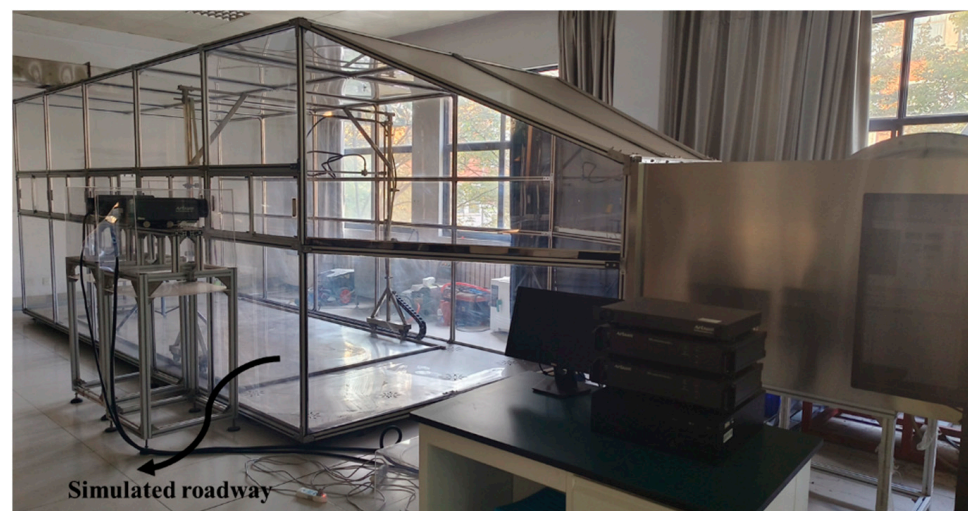
Figure 3. Airflow dust coupling test platform.
