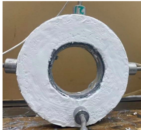
Figure 16. Test diagram of disc assembly for air cooling test.
