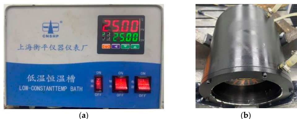
Figure 8. Cooling system: (a) Chiller; (b) Cooling water jacket.
