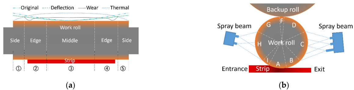
Figure 4. Boundary conditions of the work roll: (a) lateral partition; (b) circumferential cooling conditions.
