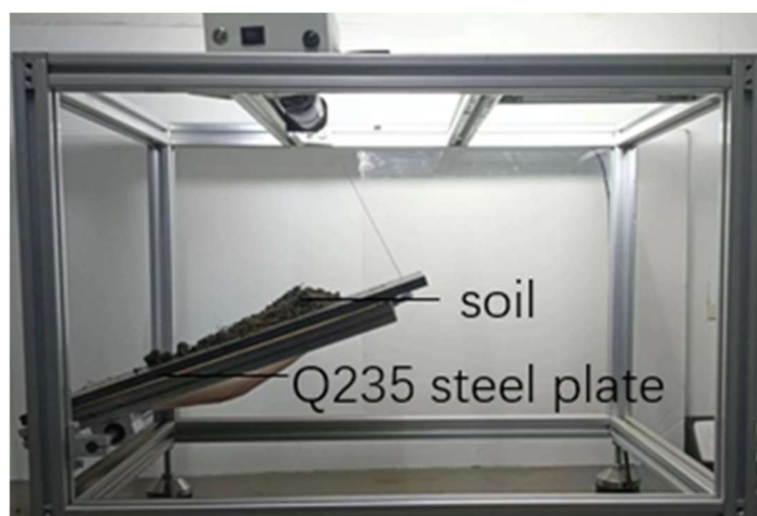
Figure 5. Physical test of sliding friction angle.
