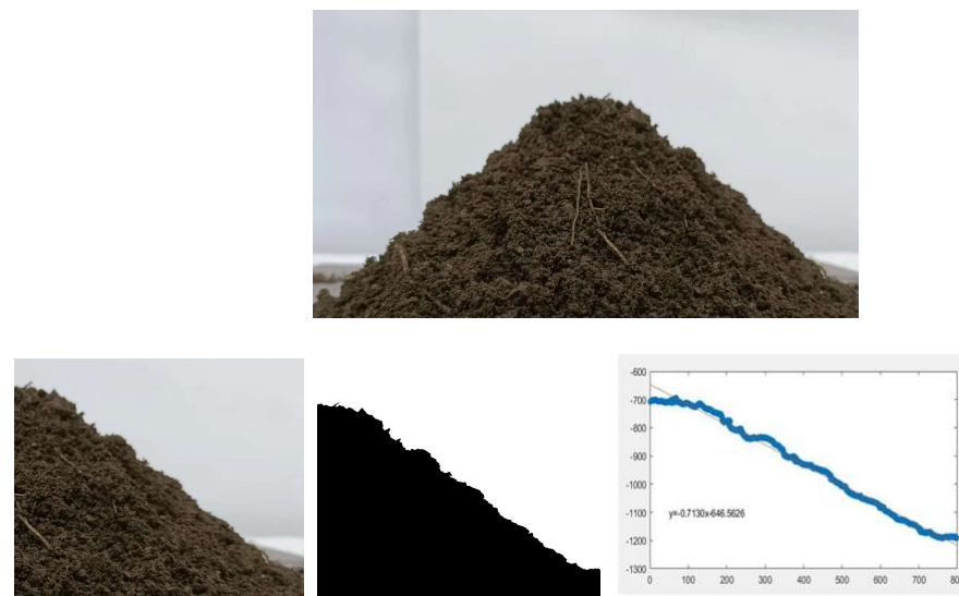
Figure 4. Physical experiment of soil accumulation.
