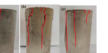
Figure 3. Compressive strength test results. (a) shear failure, (b) undergoes crush, (c) delamination failure.
