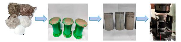
Figure 2. Flow chart of compressive strength experiment.
