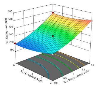
Figure 5. Factor interactions on slurry setting time.
