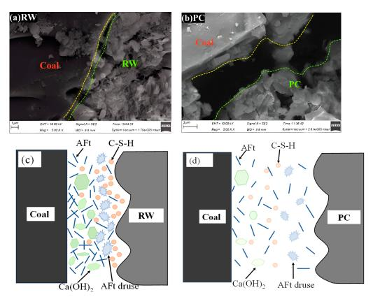
**Figure 9.** ITZ microstructure of different concretion samples. (**a**) microscopic morphology of the slurry—coal transition zone of RW material, (**b**) microscopic morphology of the slurry—coal transition zone of PC material, (**c**) schematic diagram of hydration process in slurry—coal transition zone of RW material, (**d**) schematic diagram of hydration process in slurry—coal transition zone of PC material.
