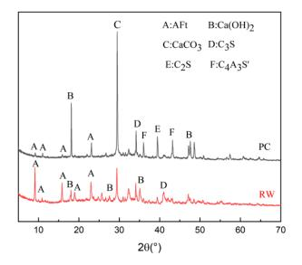
Figure 1. Physical composition analysis of basic materials.
