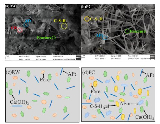
**Figure 8.** Hydration products of different grouting materials. (**a**) microstructure of RW material, (**b**) microstructure of PC material, (**c**) schematic diagram of the microscopic hydration process of RW material, (**d**) schematic diagram of the microscopic hydration process of PC material.
