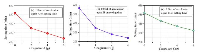
Figure 4. Effect of type and dosage of coagulants on setting time of RW materials.
