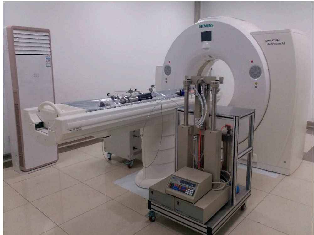
Figure 2. Coreflooding system, including CT scanner, core holder, and Isco pump.
