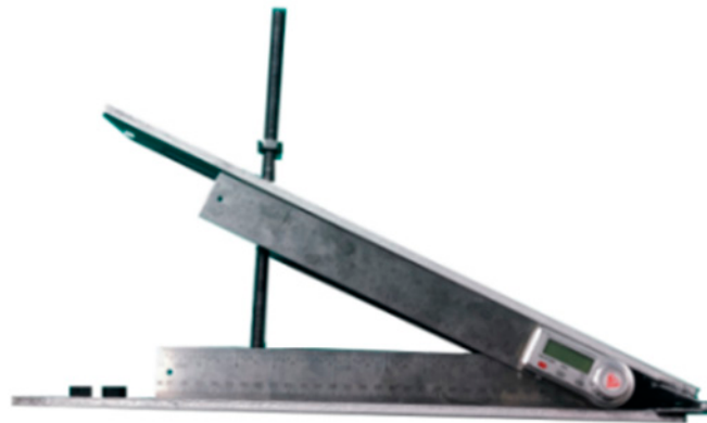
Figure 3. Home-made inclined plane instrument.
