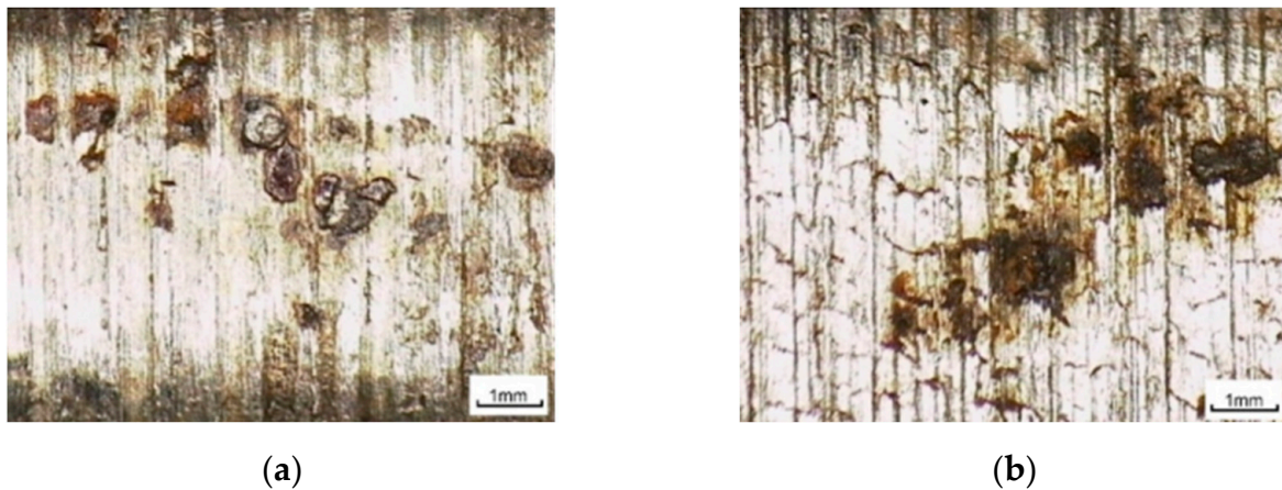
Figure 6. Optical micrograph of locally corroded surface: (a) 4330; (b) 30CrMoA (magnification: 200 \times ).
