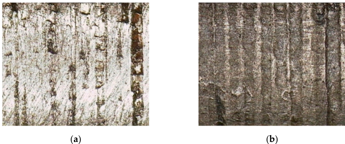
Figure 11. Surface optical micrograph of 4142 specimen before and after corrosion (magnification: 180\times ): (a) surface before corrosion; (b) surface after corrosion.
