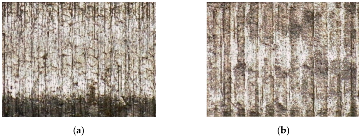
Figure 10. Surface optical micrograph of 20CrMoA specimen before and after corrosion (magnification: 180\times ): (a) surface before corrosion; (b) surface after corrosion.
