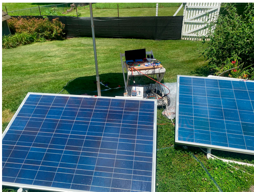
Figure 2. A PV/T system utilized to validate the mathematical model.
