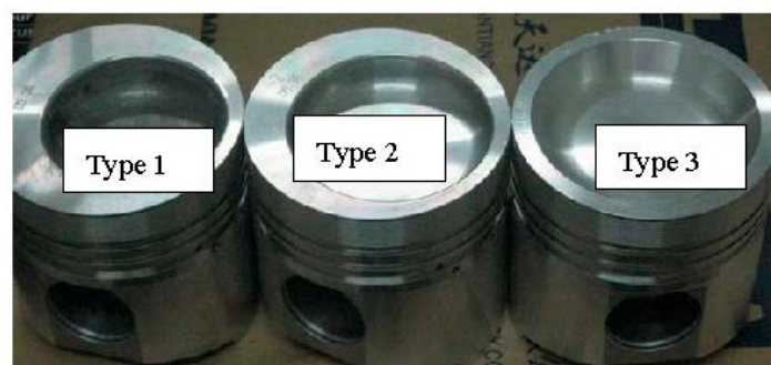
Figure 2. Shapes of the three main combustors.
