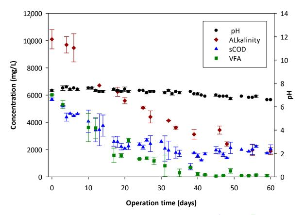
**Figure 2.** Variation of organic matter measured with sCOD ( $\blacktriangle$ ) and VFA ( $\blacksquare$ ), and variation of stability measured with pH ( $\bullet$ ) and Alkalinity ( $\blacklozenge$ ) values with their standard deviations along operation time.
