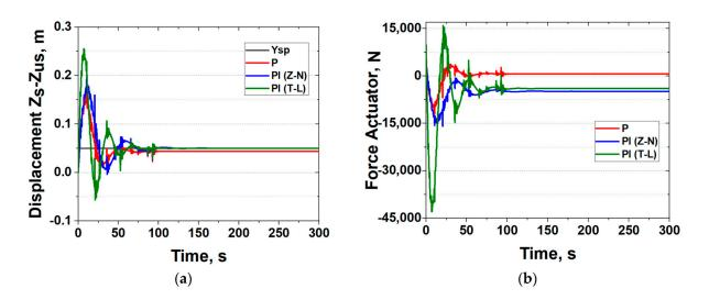
**Figure 10.** Comparison of P and PI controllers during scenario 2: (**a**) displacement of the active suspension system and (**b**) force actuator control action.
