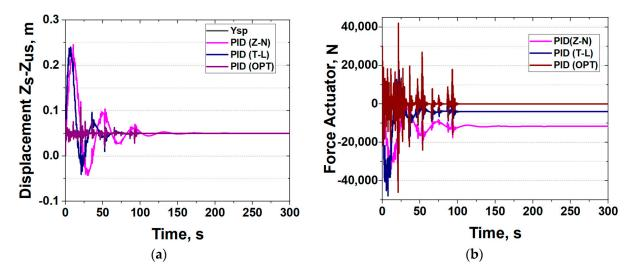
**Figure 11.** Comparison of PID controllers during scenario 2: (**a**) displacement of the active suspension system and (**b**) force actuator control action.
