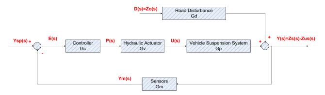
Figure 5. Feedback control for the active suspension system.
