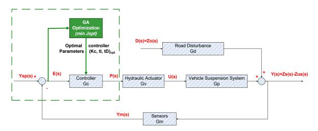
Figure 7. Optimal tuning methodology for PID controllers.
