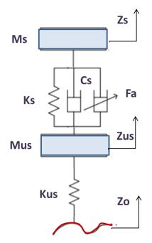
**Figure 2.** Active suspension system of a (1/4) quarter car.
