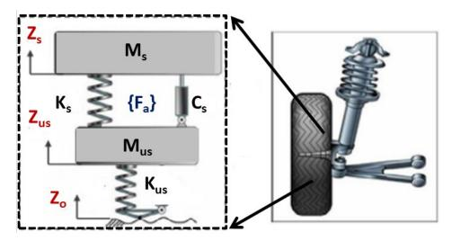
Figure 1. A quarter-car model of the suspension system.
