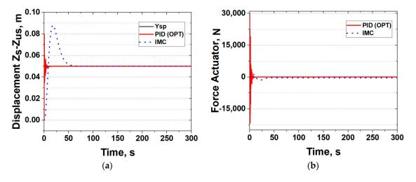
**Figure 12.** Comparison of optimal PID and IMC controllers during scenario 1: (**a**) displacement of the active suspension system and (**b**) force actuator control action.
