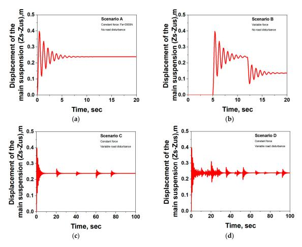
**Figure 4.** Open loop simulations for scenarios A–D: displacement of the suspension system as  $y = Z_s - Z_{us}$  (a) constant force without disturbance, (b) variable force without disturbance, (c) constant force with short-term disturbance and (d) constant force with long-term disturbance.
