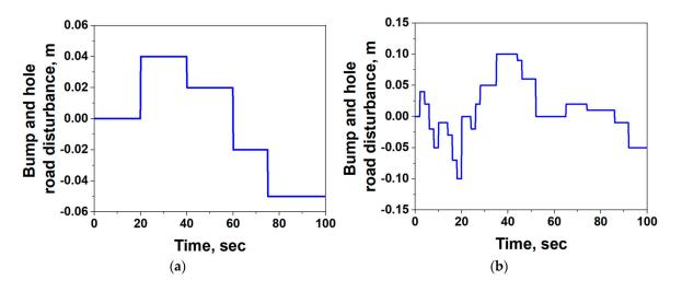
Figure 3. Bump and hole road disturbance (road anomaly) (a) short-term and (b) long-term.
