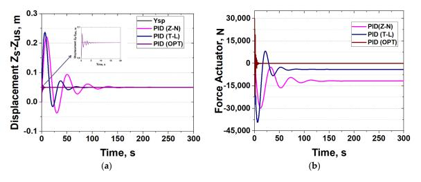
**Figure 9.** Comparison of PID controllers during scenario 1: (**a**) displacement of the active suspension system and (**b**) force actuator control action.
