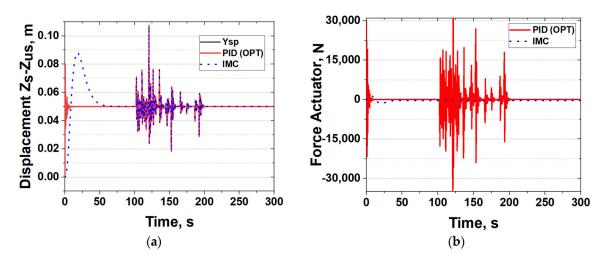
**Figure 13.** Comparison of optimal PID and IMC controllers during modified scenario 2: (**a**) displacement of the active suspension system and (**b**) force actuator control action.
