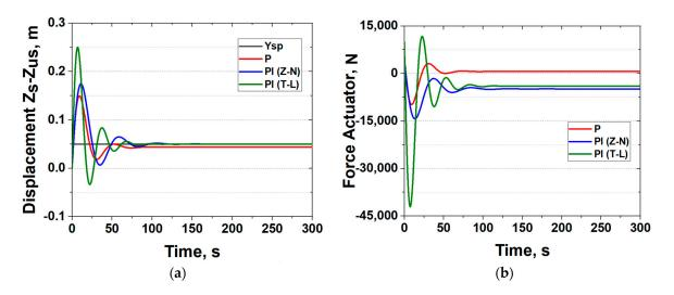
**Figure 8.** Comparison of P and PI controllers during scenario 1: (**a**) displacement of the active suspension system and (**b**) force actuator control action.
