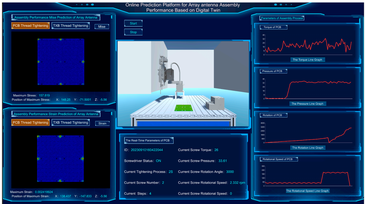
Figure 10. Performance prediction and visualization of array antenna assembly based on DT.
