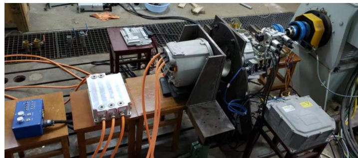
Figure 12. Test bench layout for the single-axis parallel hybrid electric vehicle.
