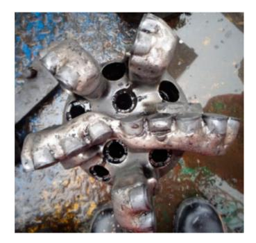
Figure 8. PDC bit after starting drilling.
