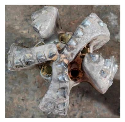
Figure 11. WS503HKPDC drill bit after drilling out.
