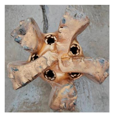
Figure 10. WS503HK PDC drill bit.
