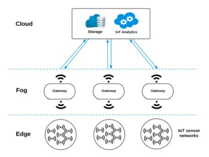
Figure 2. The architecture of the low-cost real-time monitoring system for electric motors [72].
