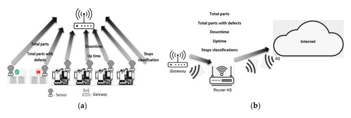
**Figure 4.** The interface between the three layers: (**a**) Monitoring of downtime, running time, and total parts with and without defects produced; (**b**) Gateway interface with the cloud layer.
