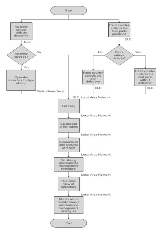
Figure 5. Flowchart describing how the system works.
