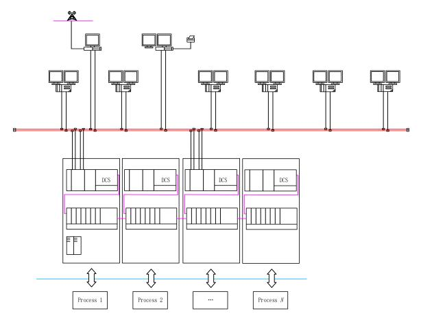
Figure 6. The workshop control station and central control room via the network bus of the control system.
