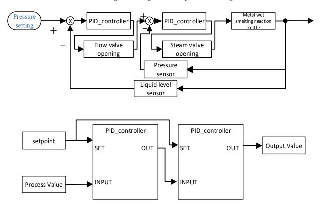
Figure 8. Reactor control.
