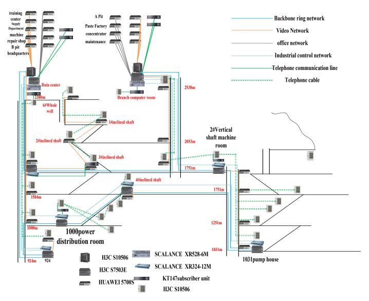
Figure 1. Underground deep metal mining network.
