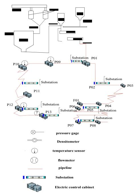
**Figure 3.** Schematic diagram of filling pipeline network control system.
