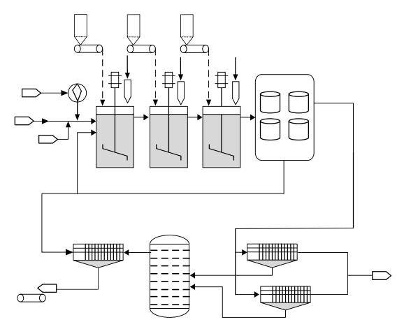
Figure 7. Complex Flotation Process of Metal Mines.
