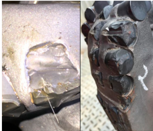
Figure 1. Abnormal failure forms such as PDC tooth breakage and delamination. (Scale on the left: 2:1).
