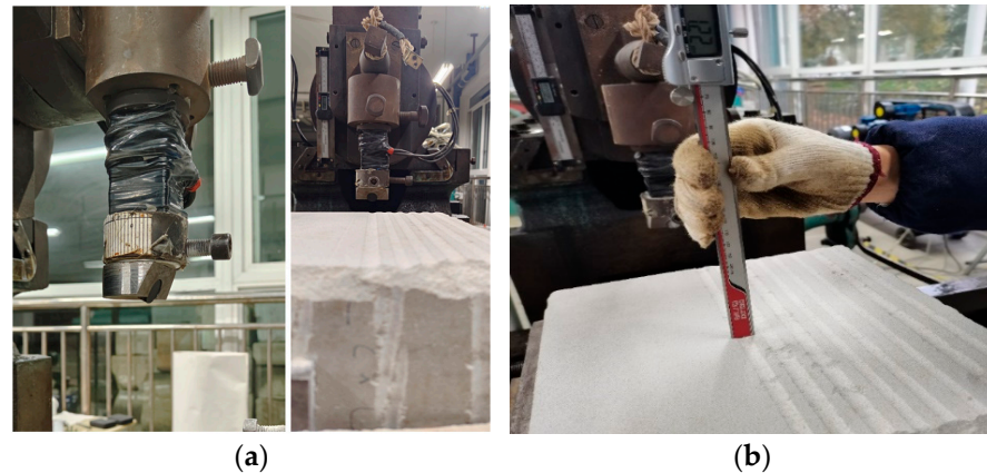
Figure 9. Part of the operation process. (a) Installation of gear seat (b) Measurement of cutting depth.
