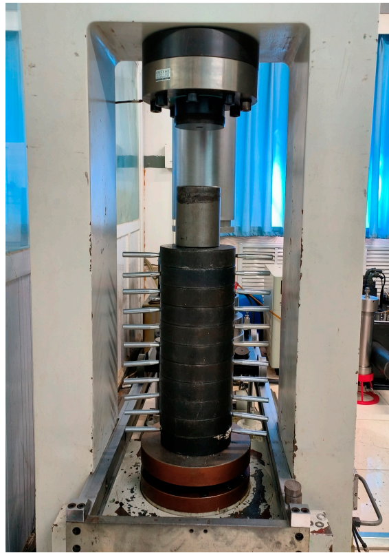
Figure 2. TAR-1500 hydraulic servo experimental test system.
