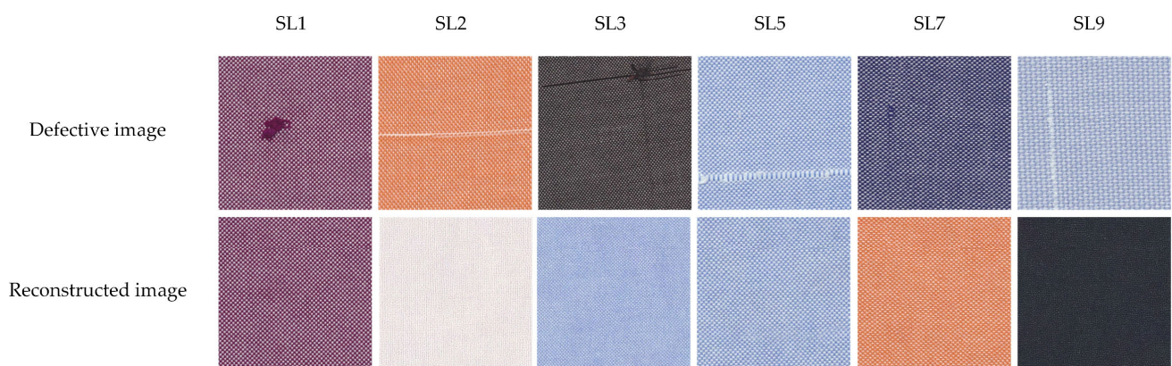
Figure 11. Model failure experiment: 19 types of defect-free fabric samples are trained and partial defect images are tested.
