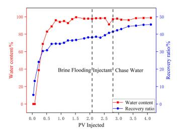
Figure 10. Core oil displacement results of nano No. 4.
