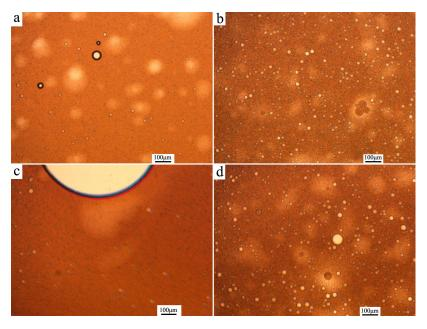
**Figure 2.** Emulsification photo of different oil displacement systems with concentration of 0.3%: (a) nano No. 1; (b) nano No. 2; (c) nano No. 3; (d) nano No. 4.
