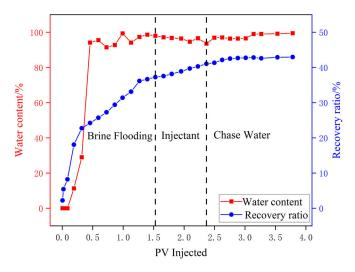
Figure 7. Core oil displacement results of nano No. 1.
