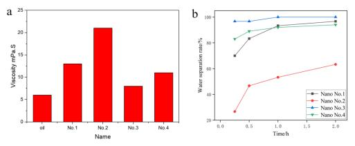
**Figure 3.** Emulsification performance of different oil displacement systems with concentration of 0.3%: (a) viscosity; (b) demulsification rate.
