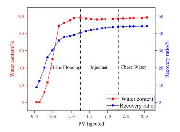
Figure 8. Core oil displacement results of nano No. 2.
