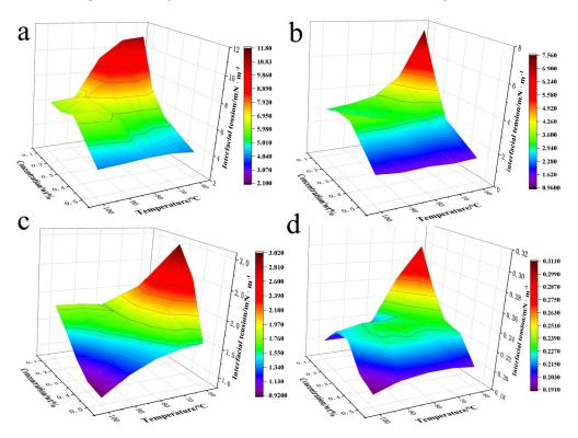
**Figure 1.** Effect of temperature and concentration of nano-oil displacement agent on oil-water interfacial tension: (**a**) nano No. 1; (**b**) nano No. 2; (**c**) nano No. 3; (**d**) nano No. 4.
