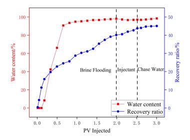
Figure 9. Core oil displacement results of nano No. 3.
