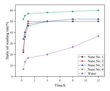
Figure 4. Static oil washing rate of different oil displacement systems with 0.3% concentration.
