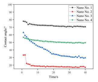
**Figure 5.** Comparison of contact angles of different nano-oil displacement agents with concentration of 0.3%.
