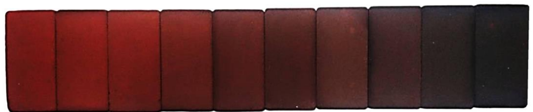
Figure 2. Image of the different families of prismatic specimens co-formed with brick dust and biomass ash. From left to right: Family A, Family B, Family C, Family D, Family E, Family F, Family G, Family H, Family I and Family J.
