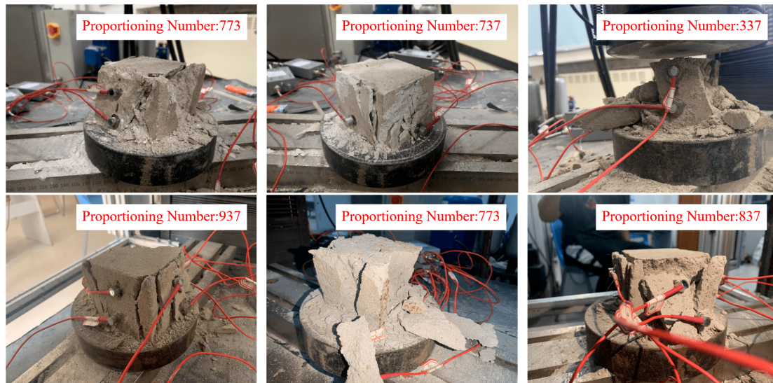
Figure 5. Uniaxial compression tests of specimens with different proportioning schemes.
