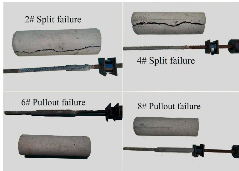
Figure 6. Damage pattern of specimen in grouted rockbolt systems.
