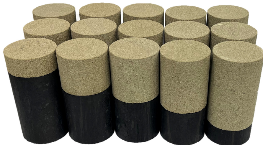
Figure 4. Soft rock–coal combinations of different height ratios.
