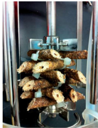
Figure 1. PCS grid setup in bioreactor.
