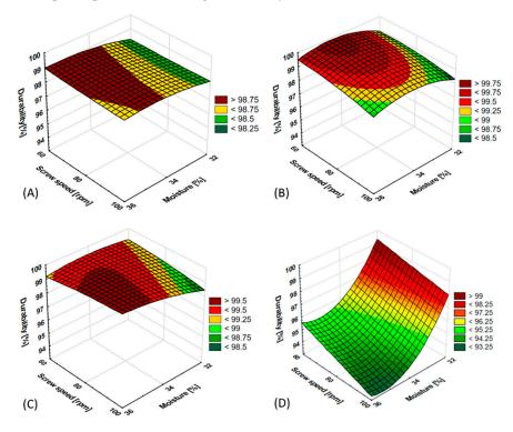
**Figure 6.** Results of durability testing of snack pellets without and with the addition of insect flour, depending on initial moisture content and applied screw speed: (**A**)control, (**B**) 10% insect powder, (**C**) 20% insect powder, (**D**) 30% insect powder.
