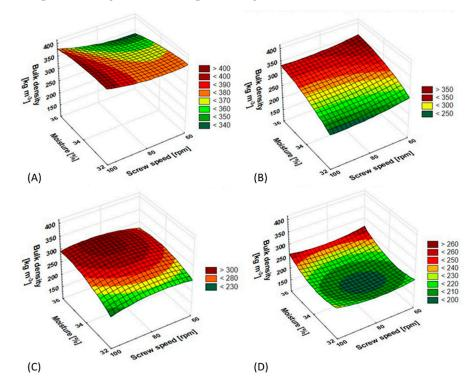
**Figure 5.** Results of bulk density testing of snack pellets without and with the addition of insect flour, depending on initial moisture content and applied screw speed: (**A**) control, (**B**) 10% insect powder, (**C**) 20% insect powder, (**D**) 30% insect powder.
