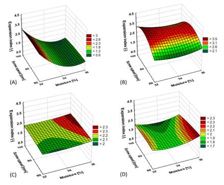
**Figure 4.** Results of expansion index testing of snack pellets without and with the addition of insect flour, depending on initial moisture content and applied screw speed: (**A**) control, (**B**) 10% insect powder, (**C**) 20% insect powder, (**D**) 30% insect powder.
