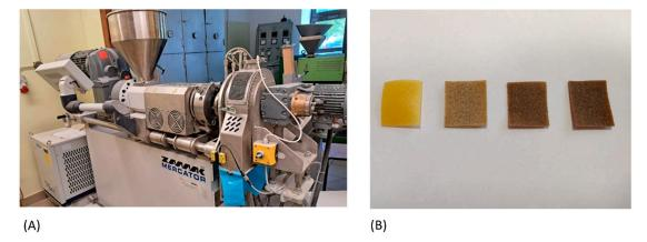
**Figure 1.** The single-screw prototype modular extruder EXP-45–32 (**A**) with L/D = 20 configuration design for snack pellet processing, and samples of the obtained snack pellets (**B**). From left: control and supplemented with 10, 20 and 30% of edible cricket flour.
