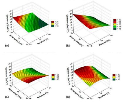
**Figure 2.** Results of snack pellet processing efficiency assessment of the tested blends without and with the addition of insect flour depending on initial moisture content and applied screw speed: **(A)** control, **(B)** 10% insect powder, **(C)** 20% insect powder, **(D)** 30% insect powder.
