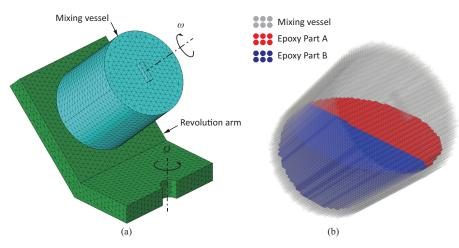
**Figure 2.** Three-dimensional particle discretization: (**a**) original meshed CAD model and (**b**) post-processed SPH particle model.
