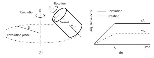
**Figure 1.** (a) Schematic of revolution–rotation planetary mixer with cylindrical vessel and (b) its operational velocity–time plot.
