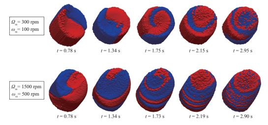
**Figure 7.** Comparison of low- and high-speed blending characteristics between Case 4 ( $\Omega_{ss}$  = 300 rpm,  $\omega_{ss}$  = 100 rpm) and Case 19 ( $\Omega_{ss}$  = 1500 rpm,  $\omega_{ss}$  = 500 rpm) in terms of the results at the initial mixing stage.
