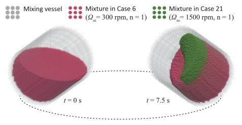
**Figure 8.** Comparison of inclination of fluid free surfaces between Case 6 ( $\Omega_{ss}$  = 300 rpm,  $\omega_{ss}$  = 300 rpm) and Case 21 ( $\Omega_{ss}$  = 1500 rpm,  $\omega_{ss}$  = 1500 rpm) at *t* = 7.5 s
