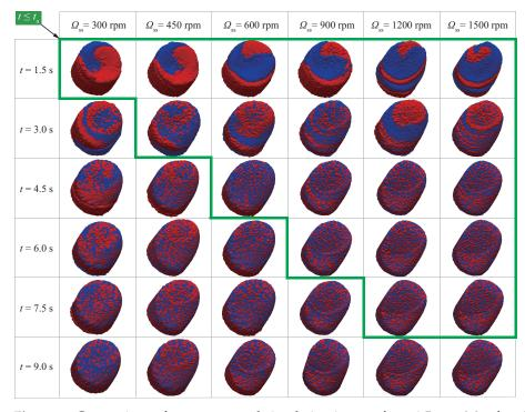
**Figure 5.** Comparison of post-processed simulation images from 1.5 s to 9.0 s for six rotational velocities with rotation-to-revolution speed ratios of 1/3.
