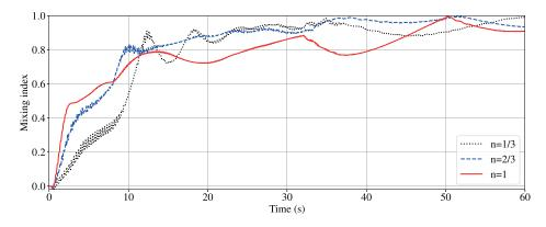
**Figure 4.** Mixing index–time curves at revolution velocity of 150 rpm with rotation-to-revolution speed ratios of 1/3, 1/2, and 1.
