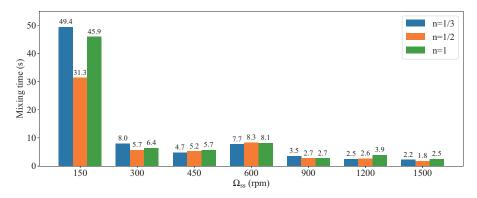
Figure 10. Bar chart of 90% mixing time for 21 simulation cases.
