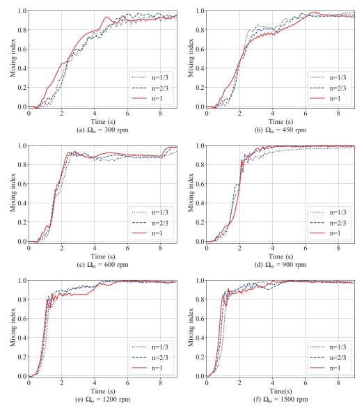
**Figure 6.** Mixing index–time curves for six rotational velocities with rotation-to-revolution speed ratios of 1/3, 1/2, and 1 for each case: (a) 300 rpm, (b) 450 rpm, (c) 600 rpm, (d) 900 rpm, (e) 1200 rpm, and (f) 1500 rpm.
