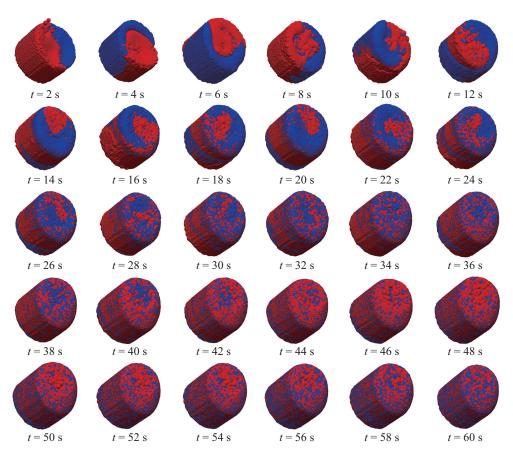
**Figure 3.** Simulation graphics for Case 1 ( $\Omega_{ss}$  = 150 rpm,  $\omega_{ss}$  = 50 rpm) from 2 s to 60 s.
