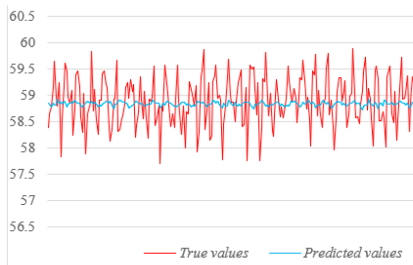
Figure 14. Stator core temperature prediction results (Stator overload).
