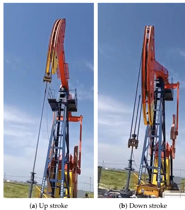
Figure 2. The operation of the pumping unit.
