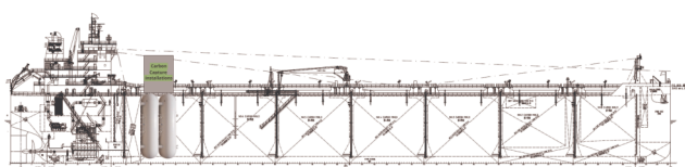
Figure 13: An arrangement for the storage on the cargo hold and some of the capture process in the hatch area in the cost of sacrificing almost 3.5-10.0% of the cargo capacity.
