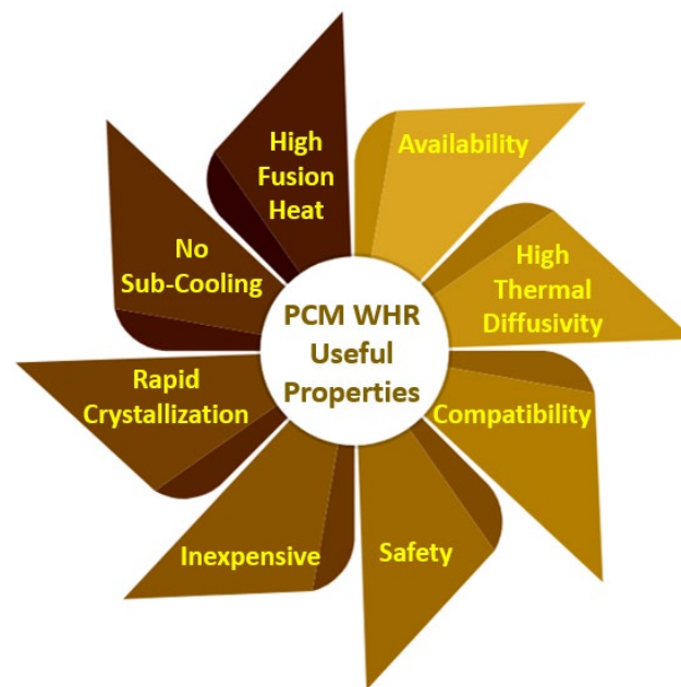
Figure 6. Phase change material characteristics of interest for waste heat recovery.
