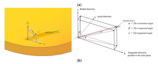
**Figure 2.** Combustor liner with tangential effusion cooling holes. (**a**) 3D model of the combustor liner. (**b**) Structure and definition of the tangential effusion cooling hole.
