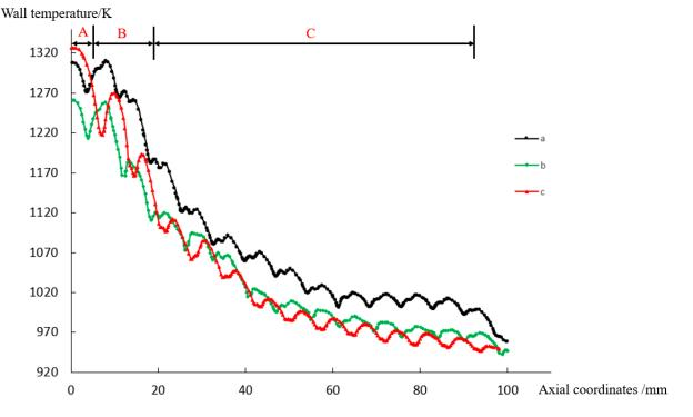
**Figure 11.** Inner wall temperature along the axial direction under the three different cooling hole arrangements.
