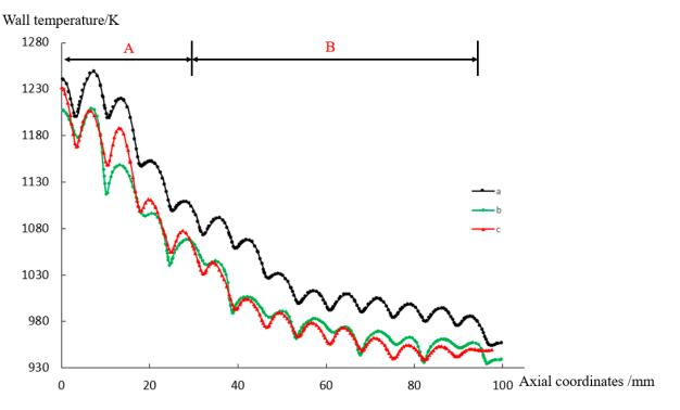
**Figure 12.** Outer wall temperature along the axial direction under the three different cooling hole arrangements.
