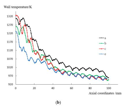
**Figure 18.** Distribution of the wall temperatures on the inner and outer wall under the improved cooling hole arrangement and the original three arrangements: (**a**) inner wall; and (**b**) outer wall.
