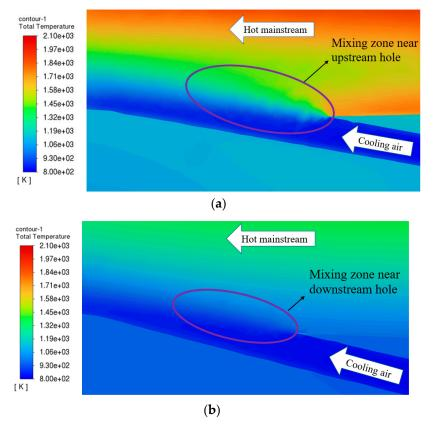
Figure 7. Heat exchange at the upper lip of the cooling hole exit.
