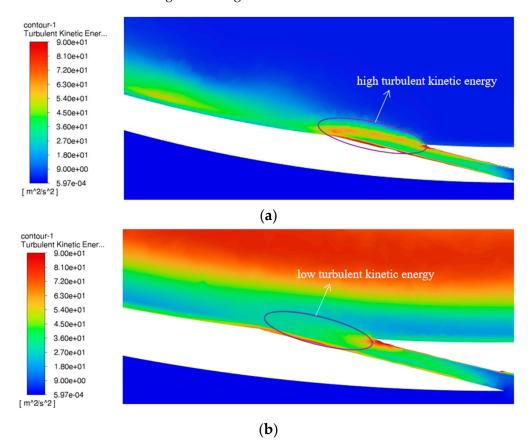
**Figure 8.** The turbulent kinetic energy around the cooling hole exit: (**a**) hole at the 4th row; and (**b**) hole at the 11th row.
