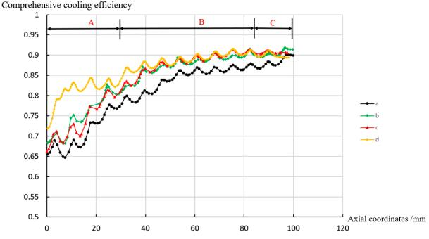
Figure 16. Comparison of the comprehensive cooling efficiencies for the liner wall under the improved cooling hole arrangement and the original three arrangements.
