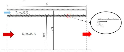
Figure 1. Schematic of the physical model.
