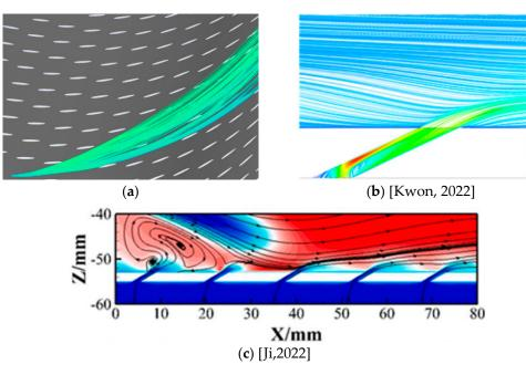
**Figure 5.** Pathlines from effusion holes. (a) Pathlines from the tangential effusion cooling hole in the present study. (b) Pathlines from the conventional effusion cooling hole in the paper by Kwon [33]. (c) Pathlines from the conventional effusion cooling holes in the paper by Ji [36].
