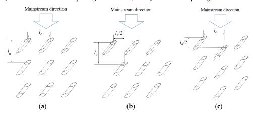
Figure 10. Three different arrangements for the cooling hole layout.
