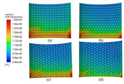
Figure 15. Temperature contours of the inner wall under the improved arrangement and the original three arrangements. (a) Arrangement "a", (b) Arrangement "b", (c) Arrangement "c", (d) Arrangement "d".
