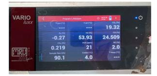
Figure 2. Gas analyzer (MRU model, Vario luxx).
