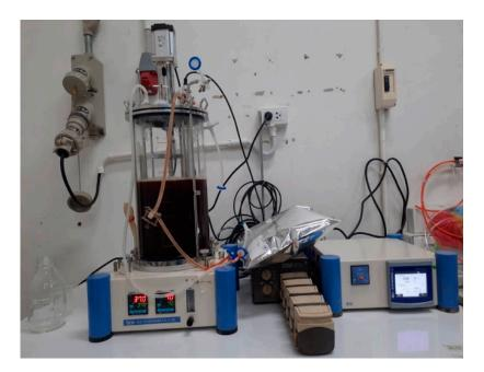
Figure 1. Ten-liter bioreactor for biohydrogen production.
