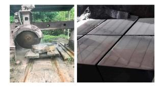
Figure 2. Process of cutting a shale outcrop.
