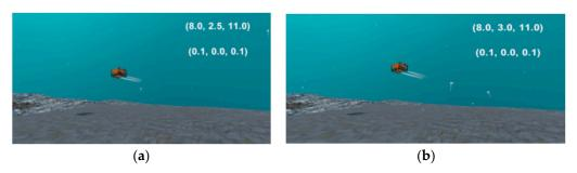
**Figure 19.** Multi-group depth target test effect. (**a**) Test effect with target depth of 2.5 m. (**b**) Test effect with target depth of 3.0 m.
