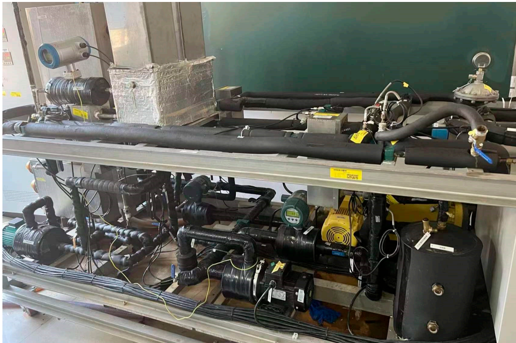
Figure 2. Single tube boiling test systems.
