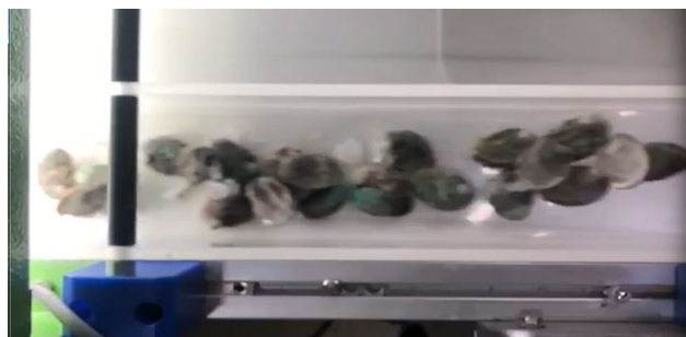
Figure 2. Entangled abalones on the conveyor belt.
