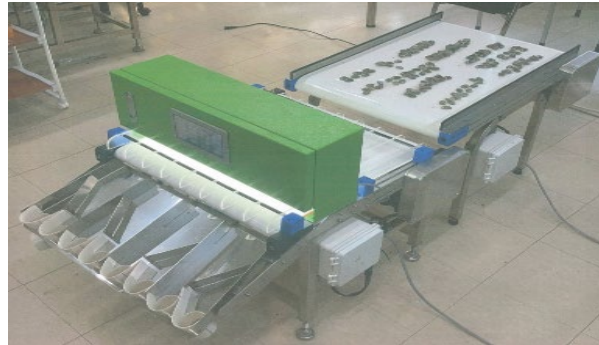
Figure 1. Abalone counting machine using conveyor belt.
