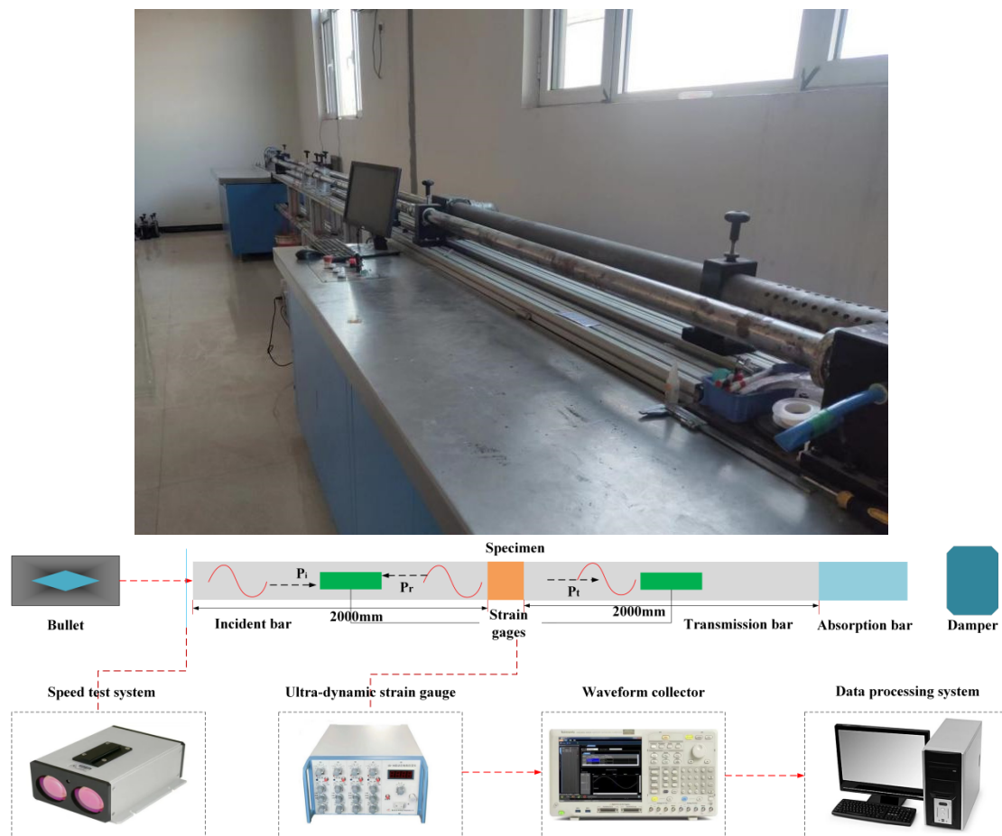
Figure 4. SHPB and schematic diagram.
