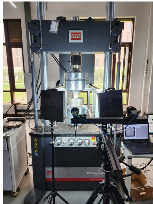
Figure 6. The Uniaxial-Compression Experimental Platform Set of MTS Experiment System and Non-Contact Whole-Strain Measurement System.
