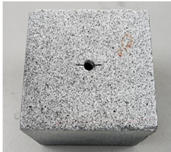
Figure 5. Shale Specimen after Spraying Speckle.
