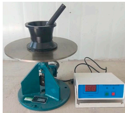
Figure 1. Flow table to determine the mortar fluidity, consistency, and setting time of cement.
