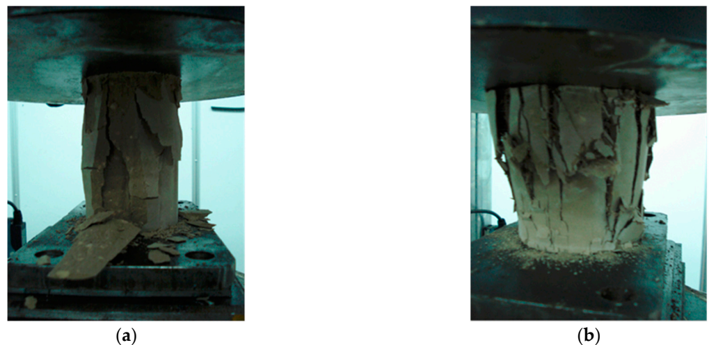
Figure 2. (a) Compression test at 1 d; (b) compression test at 3 d.
