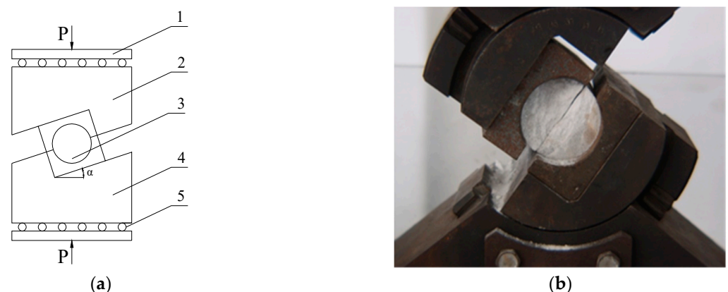
Figure 4. (a) Diagram of variable-angle shear test (1—steel spacer plate, 2—fixture upper seat, 3—test piece, 4—fixture lower seat, 5—rollers); (b) fixture of the variable-angle shear.
