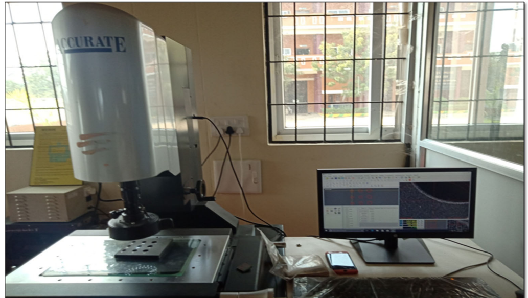
Figure 4. Profile projector vision measuring machine for the delamination of an onyx composite.
