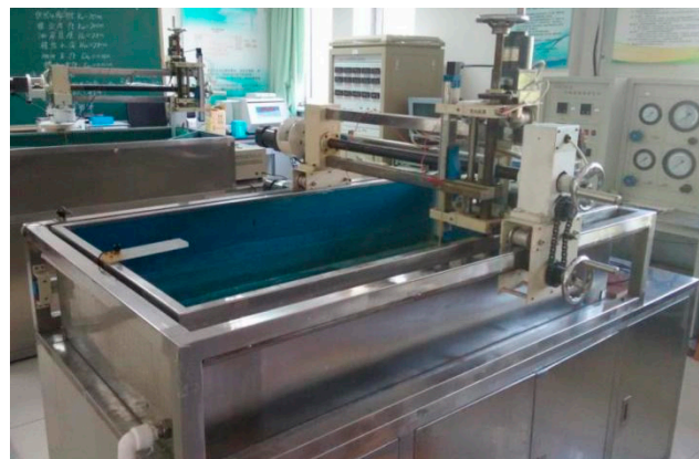
Figure 1. Electrical simulation device for fracturing corresponding to injection-production well. 1—Stabilized power supply; 2—Data collector (connected to a computer acquisition system); 3—Controller; 4—Electric motor; 5—Vertical handwheel; 6—Probe; 7—Production well; 8—Vertical cracks; 9—Horizontal handwheel; 10—Rectangular solution container.
